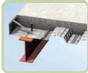
Steel - Concrete Composite Floor Beam
