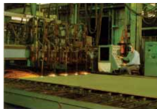
Shapecutter making multiple cuts on a clad plate.
