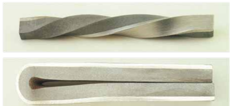
The integrity of the roll-bonded clad demonstrated by twist and bend samples.
