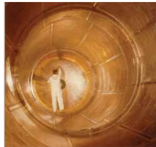
Inspecting the interior of a formed clad column.
