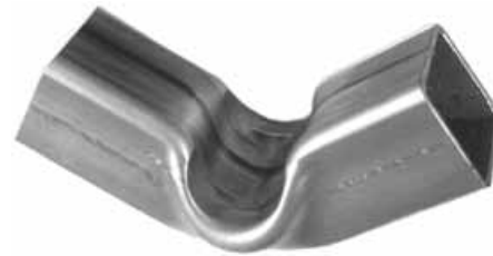
Figure 3 1/8" x 2" x 2" Duracorr ERW structural tubing transverse crush test.
