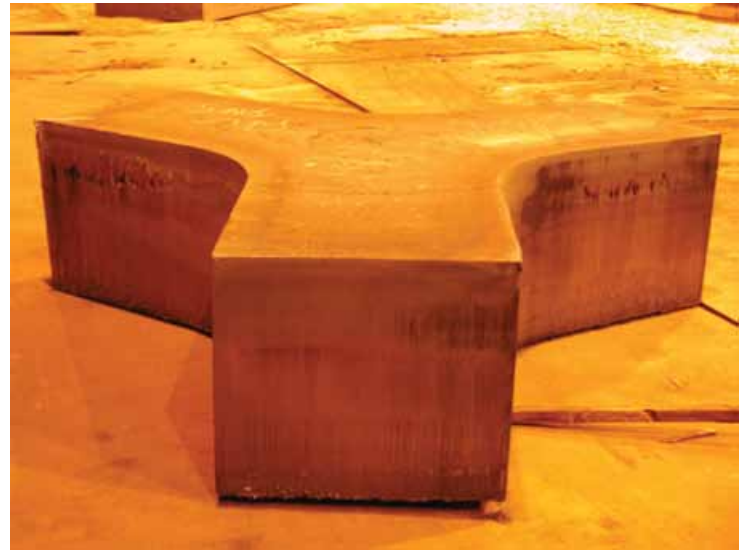
27" thick building structural element.
