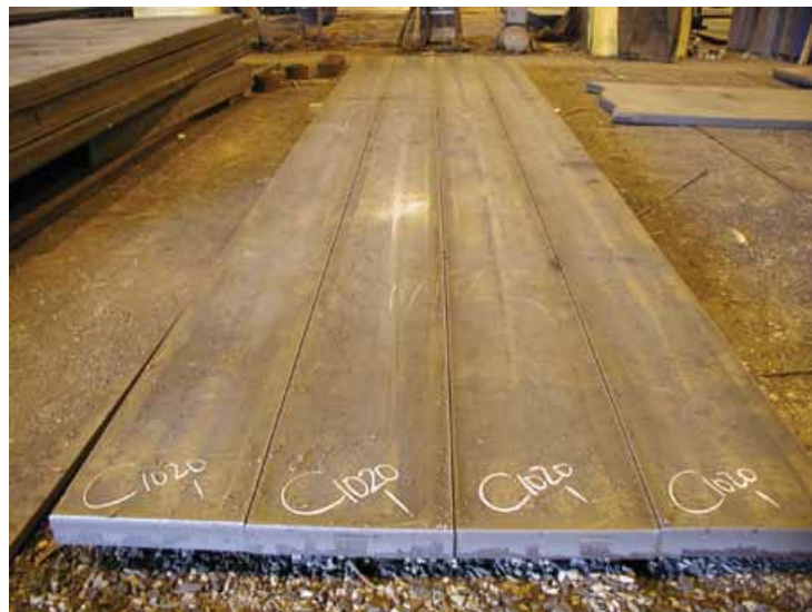
3-1/4" x 20" wide stripped plate pieces.
