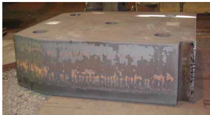
27" thick piece for machine tool press with through-holes.
