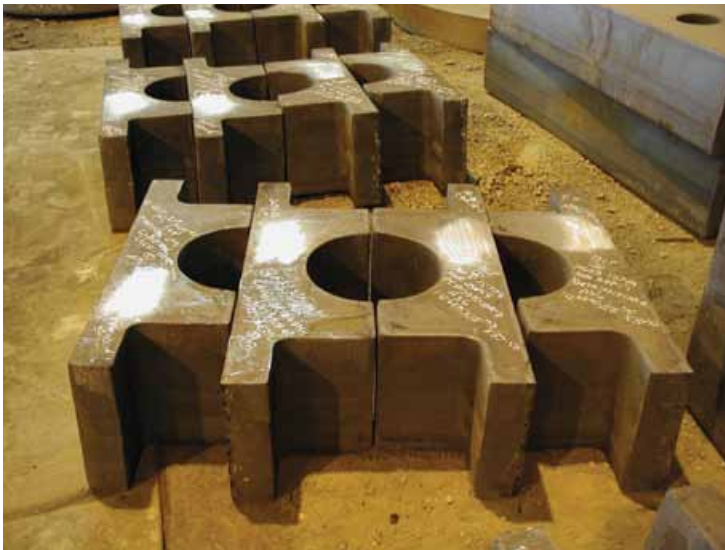
Various thick flame-cut parts including bearing blocks.
