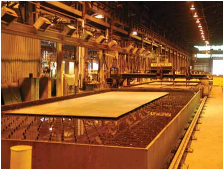
Coatesville 4-torch oxy-fuel cutting line.
