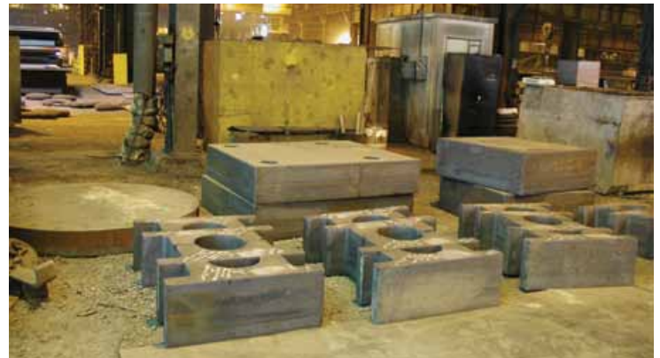
Various thick flame-cut parts including bearing blocks.
