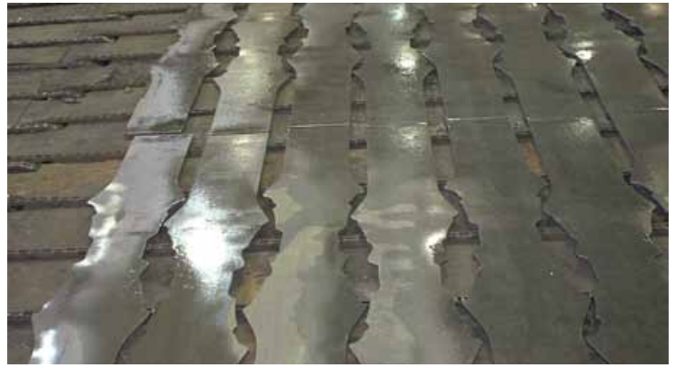
Truck axle blanks cut at Piedmont Plate Processing.
