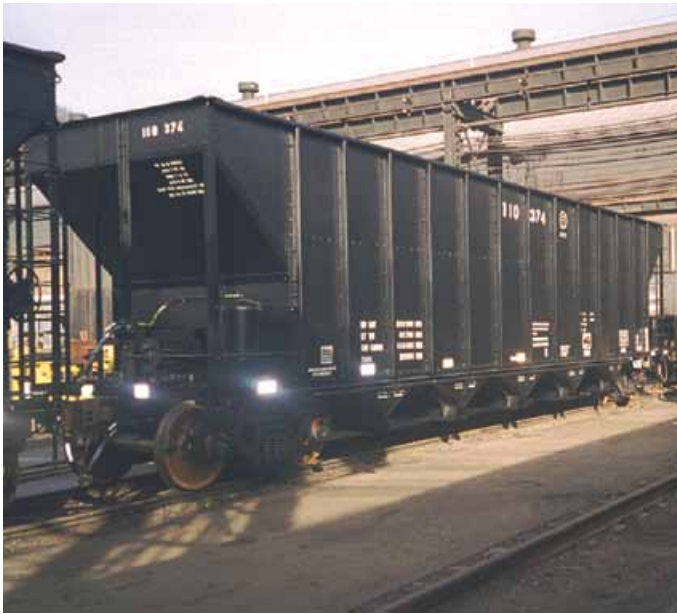
ArcelorMittal USA's Duracorr® is used in rail coal cars. The grade is Finline processed for improved toughness and formability.
