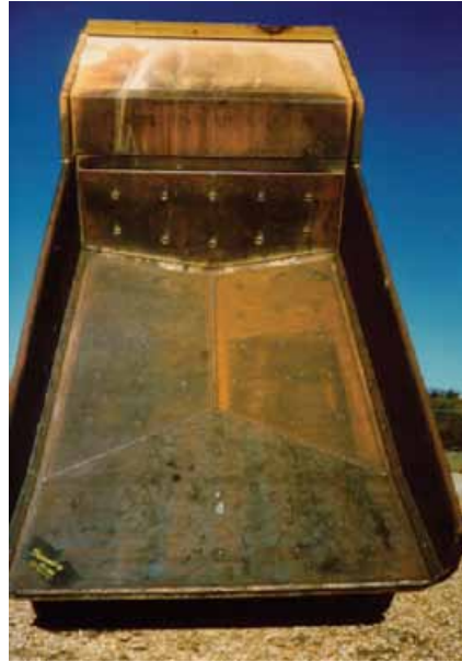
ArcelorMittal USA's Hardwear® steels are used in truck liners. Finline processing gives them improved toughness and formability.
