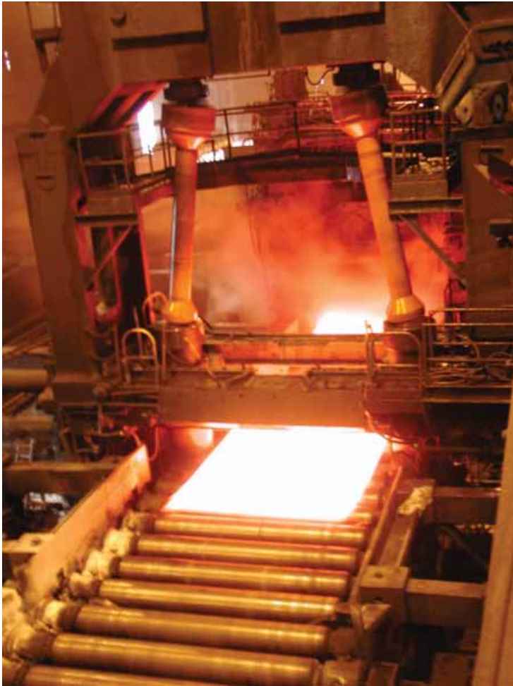
Coatesville, PA 140" Rolling Mill with vertical rolls for producing mill edge plate.
