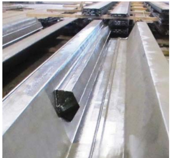
Fig. 10 Fabricated special sheet pile with inspection chamber
