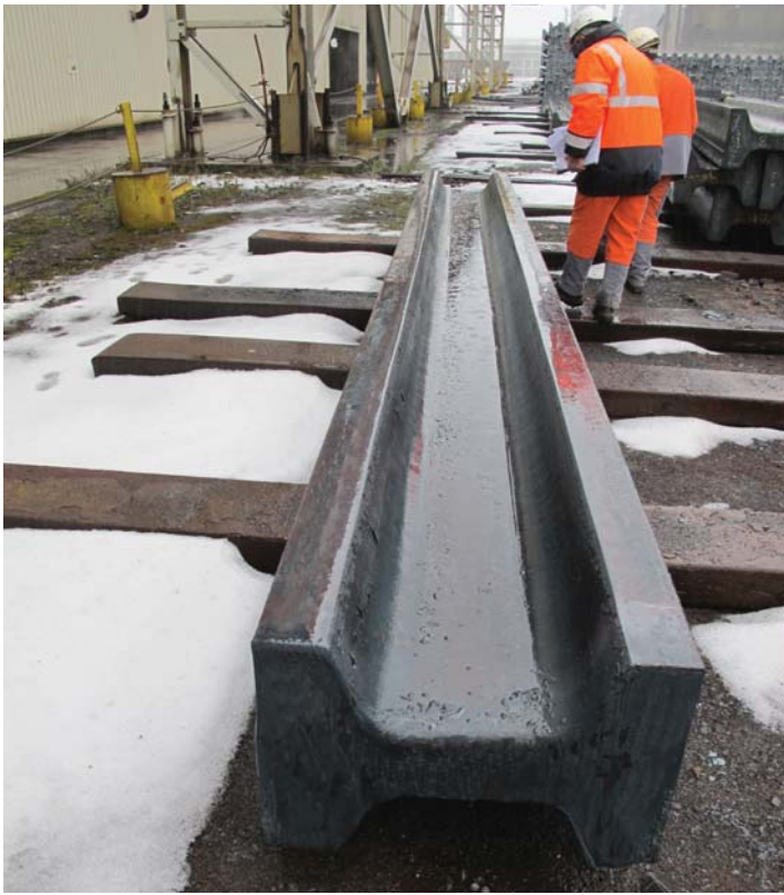
Fig. 8 AMLoCor beam blank used for rolling sheet pile
