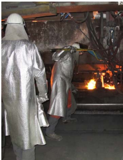
Fig. 2 Continuous casting of AMLoCor
