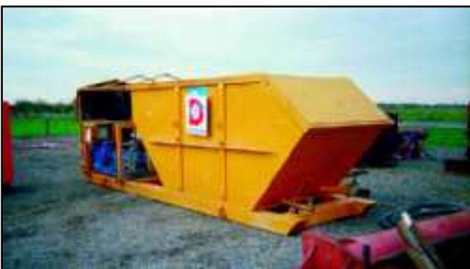
Installation with tank and pump for small project
